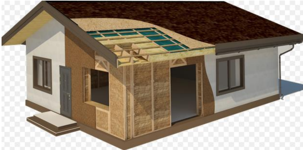
Fig.19. The design of the house using straw panels
